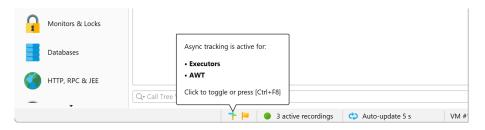
JProfiler detects if an async request tracking type that is not activated is used in the profiled JVM and shows you a ? notification icon next to the async and remote request tracking icon in the status bar. By clicking on the notification icon, you can activate the detected tracking types. Async and remote request tracking can produce substantial overhead and should only be activated if necessary.
