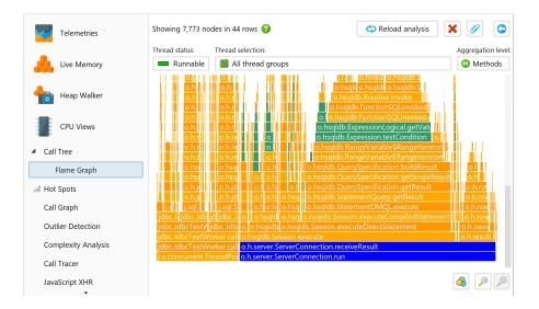
If the tool tip near the mouse cursor disturbs your analysis, you can lock it with the button in its upper right corner and then move it to a convenient location with the gripper at the top of the tool tip. The same button or a double click on the flame graph close the tool tip.
