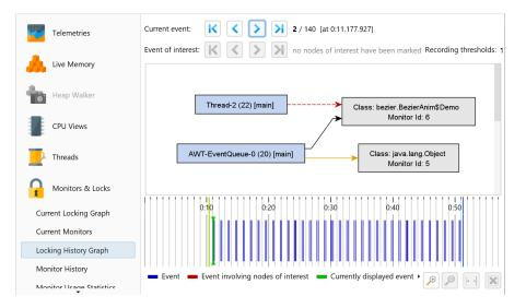
To eliminate noise and reduce memory consumption, very short events are not recorded. The view settings give you the possibility to adjust these thresholds.
