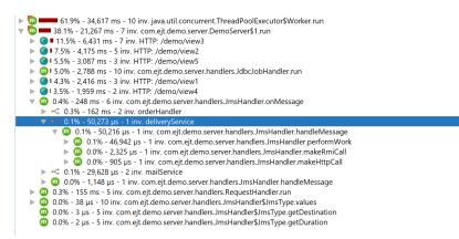
The splitting location is bound to a method, not to the selected call stack. If the same method is present somewhere else in the call tree, it will be split as well. If you use the *Merge splitting level* action, all splits will be merged into a single node. That node gives you a chance to unmerge the split again.
