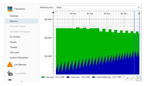
Any deeper analysis of a memory leak requires the functionality in the heap walker. To investigate a memory leak around a particular use case in detail, the "Mark heap" functionality [p. 80] is best suited. It allows you to identify new objects that have remained on the heap since a particular previous point in time. For these objects, you have to check whether they are still legitimately on the heap or if a faulty reference keeps them alive even though the object serves no further purpose.
