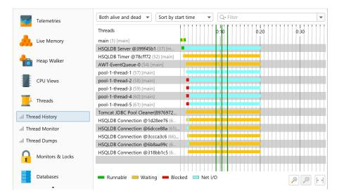
A tabular view of all threads is available in the thread monitor view. If CPU recording is active while a thread is being created, JProfiler saves the name of the creating thread and displays it
